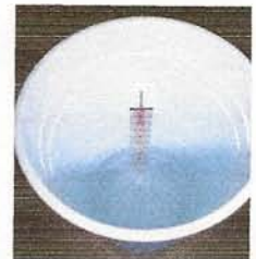
Proper Tru Blu Test strip position in cup
